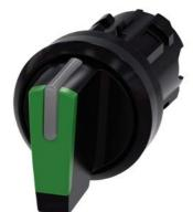
Selector switch, illuminable, 22 mm, round, plastic, green, selector switch, short, 3 switch positions I-O-II, latching, actuating angle 2x45°, 10:30h/12h/13:30h, with laser labeling, upper case and lower case, always upper case at the beginning of the word
