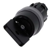
Key-operated switch O.M.R, 22 mm, round, plastic with metal front ring, lock number 73034, black, with 2 keys, 2 switch positions O<I, momentary contact type, Actuating angle 45°, 10:30h/12h, key removal O, with laser labeling, upper case and lower case, always upper case at beginning of line
