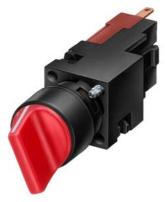
Selector switch, 16 mm, round, plastic, red, 2 switch positions O-I, latching, actuating angle 62 degree, 1 NO  $\,$
