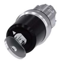
key-operated switch Siemens, 22 mm, round, metal, shiny, lock no. STGH10, with 2 keys, 2 switch positions O-I, latching, actuating angle 90°, 10:30h/13:30h, key removal O+I, with laser labeling, upper case
