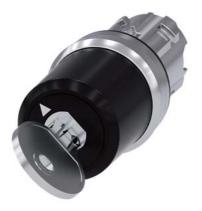
Key-operated switch BKS, 22 mm, round, metal, shiny, Lock number E1 (VW), without key, 2 switch positions O-I, latching, actuating angle 90°, 10:30h/13:30h, key removal O, with laser labeling, upper case and lower case, always upper case at beginning of line
