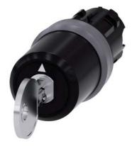
key-operated switch Siemens, 22 mm, round, plastic with metal front ring, lock number SSG10, with 2 keys, 3 switch positions I-O<II, left latching, momentary contact type on the right, actuating angle  $2x45^{\circ}$ , 10:30h/12h/13:30h, key removal O+I
