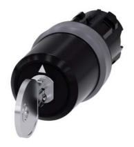
Key-operated switch BKS, 22 mm, round, plastic with metal front ring, lock number S1, with 2 keys, 3 switch positions I-O-II, latching, actuating angle  $2x45^{\circ}$ , 10:30h/12h/13:30h, key removal I, with laser labeling, lower case
