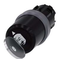
Key-operated switch BKS, 22 mm, round, plastic with metal front ring, Lock No. E7 (VW), without key, 2 switch positions O-I, latching, actuating angle 90°, 10:30h/13:30h, key removal O, with laser labeling, lower case
