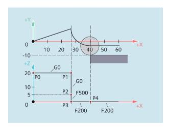
During retraction, the roles of the modally active feedrate from the previous block and the programmed feedrate value in the SAR block are reversed, i.e. the actual retraction contour is traversed with the old feedrate and a new speed programmed with the F word applies from  $P_2$  up to  $P_0$ .
