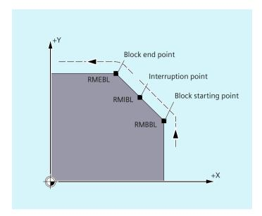
RMIBL DISPR=... or RME DISPR=... allows you to select a repositioning point which lies before the interruption point or the block end point.
