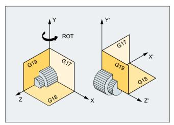
Figure 3-25 Rotation around the Y axis or in the G18 plane
