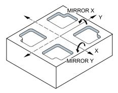
Mirroring is implemented in relation to the currently valid coordinate system set with G54 to G57, G505 to G599.
