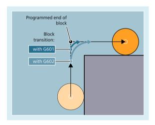
G601 activates the exact stop criterion "Exact stop fine": The block change is performed as soon as the axis-specific tolerance limits for "Exact stop fine" (MD36010 \$MA\_STOP\_LIMIT\_FINE[<Ax>]) are reached for all axes involved in the traversing motion.
