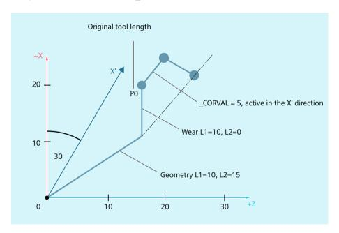
If the program example is continued after N110 with the following instructions, then the remaining wear is included completely in the geometry because the compensation is now effective in the Z' axis (parameter <GeoAx> = 0):
