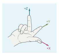
Rotary motion around the coordinate axes X, Y and Z are designated A, B and C. The direction of rotation is obtained from the direction of the rotary motion when looking in the positive direction of the coordinate axis:
