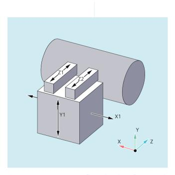
The geometry axes are configured so that after powering-up, initially Z1 is effective as 3rd geometry axis under the geometry axis name "Z" and together with X1 and Y1 forms the geometry axis group.
