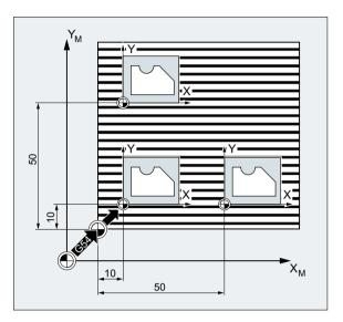
With this workpiece, the shapes shown recur in a program.
