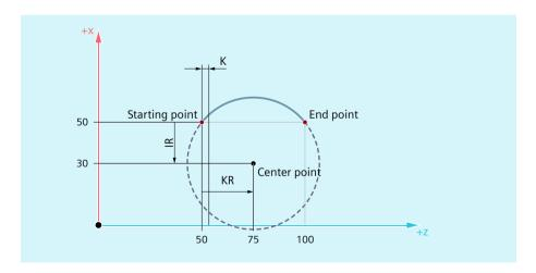
Figure 3-13 Convex thread in the clockwise direction with end and center point programming
