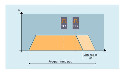
MEAWA is used for special measuring tasks in which a programmed position always has to be approached.
