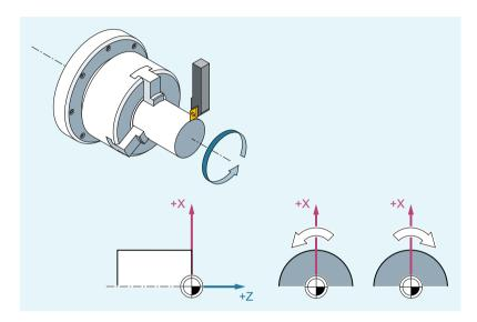
Other spindles may be available in addition to the main spindle (e.g. the counterspindle or an actuated tool on turning machines). As a rule, the main spindle is declared the master spindle in the machine data. This assignment can be changed using an NC command.
