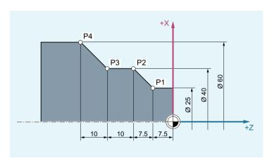
In incremental dimensions, the following position specifications are obtained for points P2 to P4:
