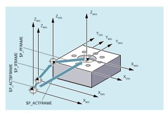
Figure 4-2 Frame variable \$P\_ACTFRAME
