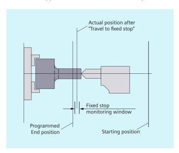
With sufficiently reduced torque, it is also possible to perform simple measurement operations without connecting a probe. The "travel to fixed stop" function can be implemented for axes as well as for spindles with axis-traversing capability.
