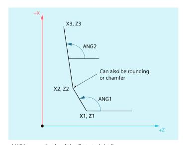
ANG1: Angle of the first straight lineANG2: Angle of the second straight lineX1, Z1: Start coordinates of the first straight line
