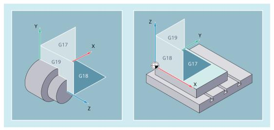
Figure 3-1 Working planes for turning and milling
