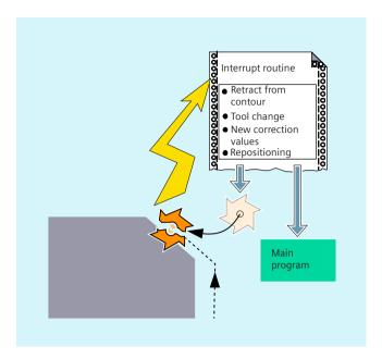
The tool breaks during machining. This triggers a signal that stops the current machining process and simultaneously starts a subprogram – known as an interrupt routine. The interrupt routine contains all the statements which are to be executed in this case.
