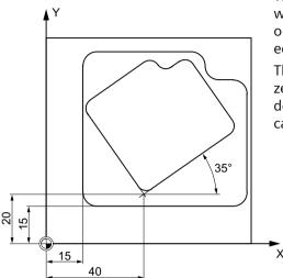
The pocket occurs twice on this workpiece, but with different sizes and rotated in relation to one another. The machining sequence is stored in the subprogram.
