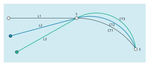
Figure 3-11 Tangentially connecting circular paths depend on the previous contour element
