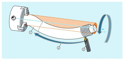
Figure 3-12 Turning a convex thread
