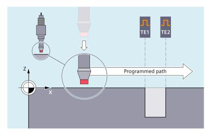
MEASA or MEAWA is used in this example to measure one drilled hole for the X axis along a programmed traversing path. The two trigger events TE1 and TE2 required for this are evaluated in the mode "one after the other in the programmed order". A contact-free switching probe is used (e.g. inductive probe).
