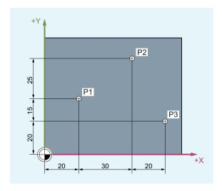
In incremental dimensions, the following position specifications are obtained for points P1 to P3:
