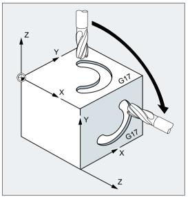
In this example, identical shapes are machined in two workpiece surfaces perpendicular to one another via subprograms. In the new coordinate system on the right-hand workpiece surface, infeed direction, working plane and the zero point have been set up as on the top surface. Therefore, the conditions required for the subprogram execution still apply: Working plane G17, coordinate plane X/Y, infeed direction Z.
