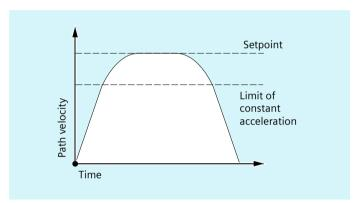
Figure 4-7 Path velocity curve with DRIVE
