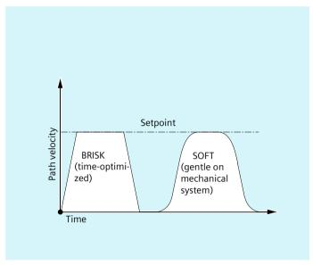
Figure 4-6 Path velocity curve with BRISK and SOFT
