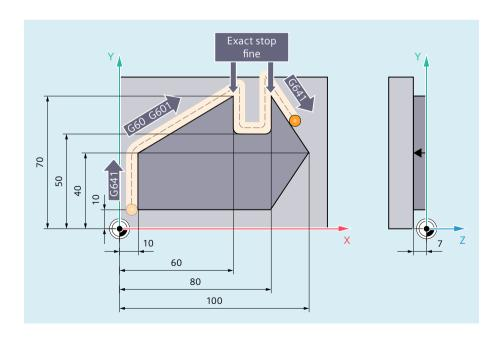
The two outside corners on the groove are to be approached exactly. Otherwise machining should be performed in continuous-path mode.
