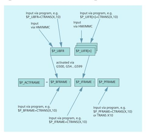
Basic frame and settable frame are effective after Reset if MD 20110 RESET\_MODE\_MASK is set as follows:
