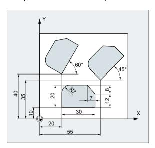
With this workpiece, the shapes shown recur in a program. In addition to the work offset, rotations have to be performed, as the shapes are not arranged paraxially.
