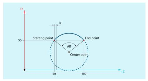
Figure 3-16 Convex thread in the clockwise direction with end point and opening angle programming
