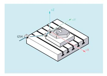
The frame components can only contain intermediate values for the description of pallet tasks. These are chained to generate various workpiece zeroes.
