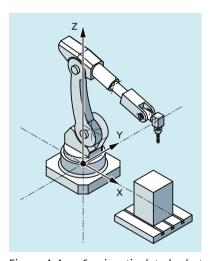
Figure 4-4 6-axis articulated robot with milling spindle
