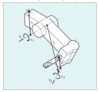
For machines with **resolved kinematics** (both the tool and the part can rotate), the system variables have been extended with the entries \$TC\_CARR18[m] to \$TC\_CARR23[m].
