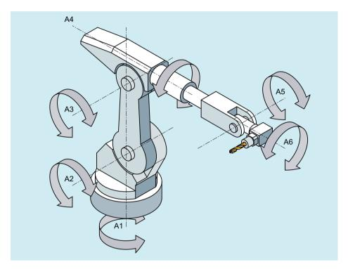
Axes A1, A2 and A3 are the main axes of the articulated robot. The axes A4, A5 and A6, which are also designated as head or hand/wrist axes, are positioned in the working area with the main axes. The additional motion options of the hand/wrist axes enable the milling spindle to be orientated in space as required for the particular machining task. Various articulated joint positions are possible to achieve the same tool orientation.
