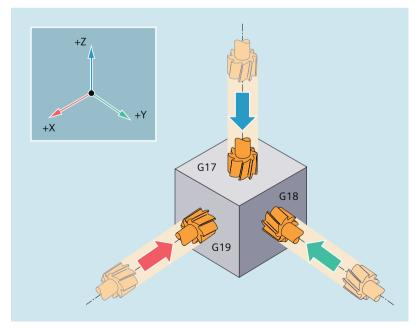
Figure 3-2 Feed directions for milling
