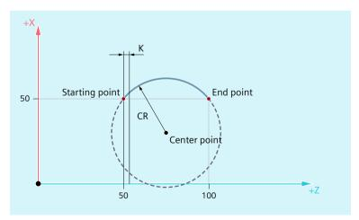
Figure 3-15 Convex thread in the clockwise direction with end point and radius programming
