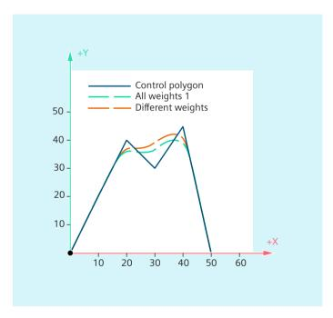
Example 2: C spline, zero curvature at the start and at the end
