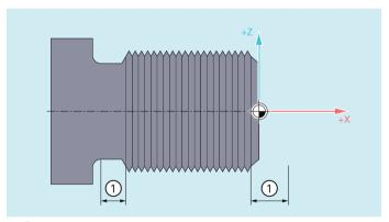
1 Run-in/run-out path, depending on the machining direction
