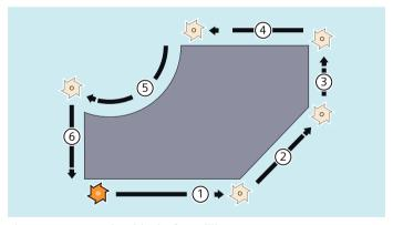
Figure 3-8 Motion blocks for milling
