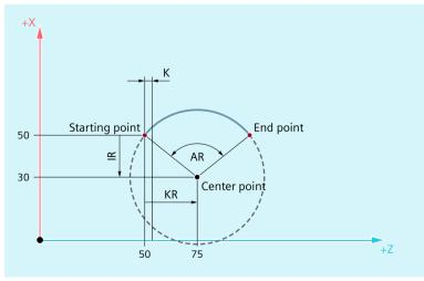
Figure 3-17 Convex thread in the clockwise direction with center point and opening angle programming
