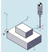
Example: Measuring a workpiece at the turning machine
