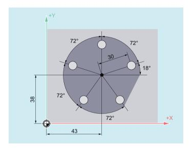
The positions of the holes are specified in polar coordinates. Each hole is machined with the same production sequence: Rough-drilling, drilling as dimensioned, reaming ...
