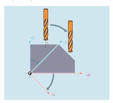
For machining inclined surfaces, the tool offsets must be appropriately defined or calculated based on the functions for "Tool length compensation for tools that can be orientated".
