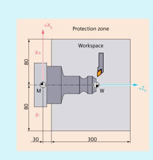
Using the working area limitation G25/26, the working area of a lathe is limited so that the surrounding devices and equipment - such as revolver, measuring station, etc. are protected against damage.
