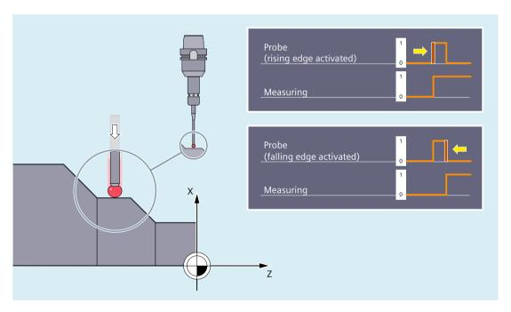
When the trigger event occurs, the positions of all traversed path and positioning axes of the block are recorded and stored in system variables.
