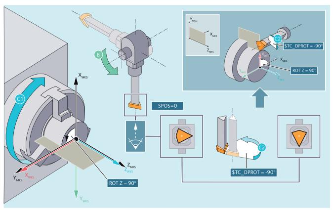
Figure 3-5 Y turning in working range 2 (WCS rotation around Z: +90°): Tool positioning via the setting angle \$TC\_DPROT
