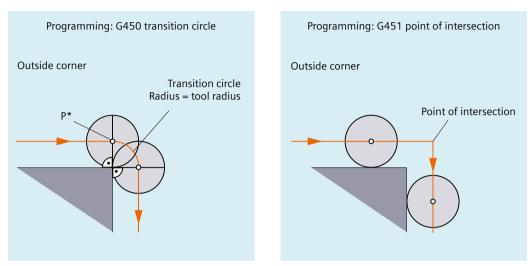
Figure 3-21 Traveling around a 90° outside corner with G450 or G451
