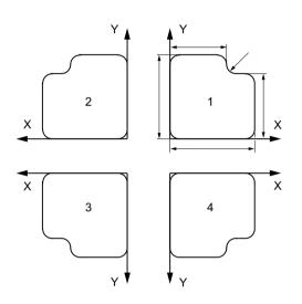
The contour shown here is programmed once as a subprogram. The three other contours are generated using mirroring. The workpiece zero is located at the center of the contours.
