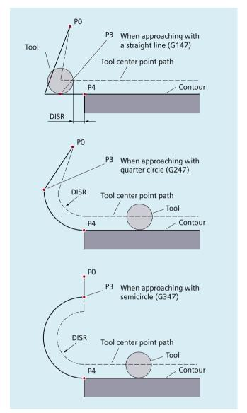
Figure 3-22 Approach movements with simultaneous activation of the tool radius compensation
