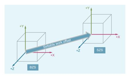
If no programmable coordinate transformations (frames) are active, then the "settable zero system" is the workpiece coordinate system (WCS).
