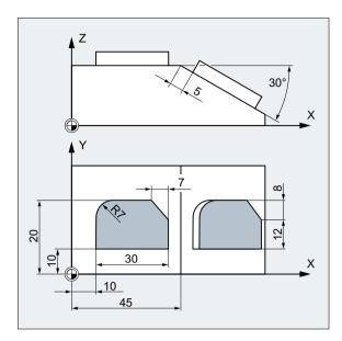
In this example, paraxial and inclined workpiece surfaces are to be machined in a clamping.
