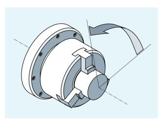
SPOS, SPOSA and M19 induce a temporary switchover to position-controlled mode until the next M3/M4/M5/M41 to M45.
