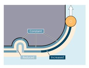
The feedrate is reduced for inside radii and increased for outside radii. This ensures a constant velocity at the tool cutting edge and thus at the contour.
