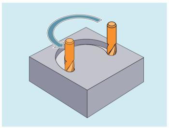
Figure 3-9 Application example: Milling a circular way
