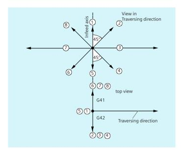
The retraction in the tool direction is defined for ALF=1.
