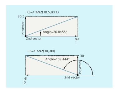
The angular reference is always based on the 2nd value in the positive direction.
