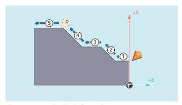
Figure 3-7 Motion blocks for turning
