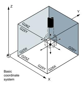
The working area limitation for all validated axes must be programmed with the WALIMON command. The WALIMOF command deactivates the working area limitation. WALIMON is the default setting. Therefore, it only has to be programmed if the working area limitation has been disabled beforehand.
