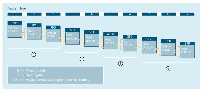
Example 4: Display response for different DISPLON/DISPLOF combinations
