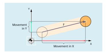
The feedrate is specified under address F. Depending on the default setting in the machine data, the units of measurement specified with the G commands are either in mm or inch.
