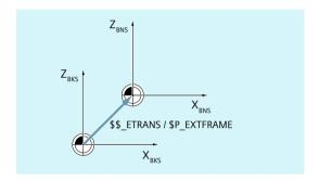
The external zero offset with \$AA\_ETRANS acts in two ways depending on the machine data parameterization:
