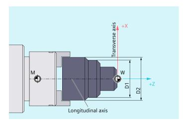
The geometry axis that is to serve as transverse axis is defined in the machine data ( $\rightarrow$  machine manufacturer).
