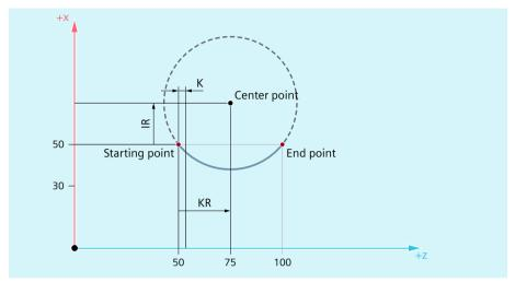
Figure 3-14 Convex thread in the counter-clockwise direction with end and center point programming
