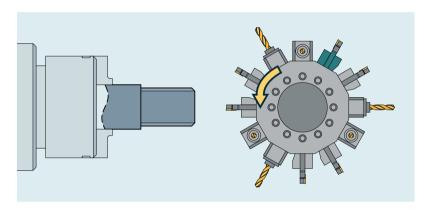
In turret magazines on turning machines, the tool change, that is the search for and change of the tool, is called with the T command only.
