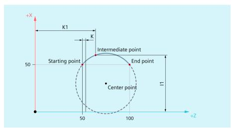
Figure 3-18 Convex thread in the clockwise direction with end and intermediate point programming
