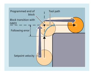
The block change is initiated when the control has calculated a set velocity of zero for the axes involved. At this time, the actual value is behind by a lag portion. The workpiece corners can now be rounded. The effect depends on the dynamic response of the axes and the path velocity:
