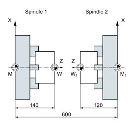
The actual machining is stored as a subprogram and execution at the respective spindle is implemented by means of mirroring and offsets.
