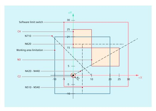
In the example, the active software limit switches and working area limits in the X-Y plane and the following three protection zones are displayed:
