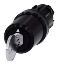
Key-operated switch BKS, 22 mm, round, plastic, lock number S1, with 2 keys, 3 switch positions I-O-II, latching, actuating angle 2x45°, 10:30h/12h/13:30h, Key removal I+O+II, with laser labeling, lower case
