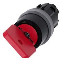
Key-operated switch O.M.R, 22 mm, round, plastic with metal front ring, lock number 73037, red, with 2 keys, 2 switch positions O<I, momentary contact type, Actuating angle 45°, 10:30h/12h, key removal O, with laser labeling, upper case and lower case, always upper case at the beginning of the word
