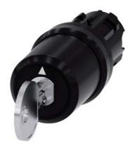
key-operated switch Siemens, 22 mm, round, plastic, special lock, with 2 keys, 3 switch positions I>O<II, momentary contact on the left, latching on the right, actuating angle 2x45°, 10:30h/12h/13:30h, key removal O
