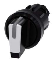
Selector switch, illuminable, 22 mm, round, plastic, white, selector switch, short, 3 switch positions I-O<II, left latching, right momentary contact type, actuating angle  $2x45^{\circ}$ , 10:30h/12h/13:30h, with laser labeling, upper case and lower case, always upper case at beginning of line
