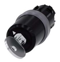
key-operated switch Siemens, 22 mm, round, plastic with metal front ring, lock no. LSG1, with 2 keys, 2 switch positions O-I, latching, actuating angle  $90^\circ, 10:30h/13:30h,$  key removal O+I, Z=50-unit packaging
