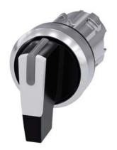
Selector switch, illuminable, 22 mm, round, metal, shiny, white, selector switch, long, 3 switch positions I-O<II, left latching, right momentary contact type, actuating angle  $2x45^{\circ}$ , 10:30h/12h/13:30h, Z=50-unit packaging
