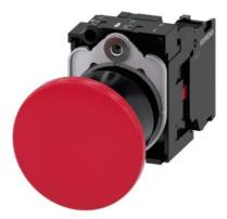
Mushroom pushbutton, 22 mm, round, plastic, red, 40mm, latching, pull-to-unlatch mechanism, with holder, 1 NC, screw terminal, with laser labeling, upper case
