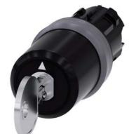
key-operated switch Siemens, 22 mm, round, plastic with metal front ring, lock number SSG10, with 2 keys, 3 switch positions I>O<II, momentary contact type, actuating angle 2x45°, 10:30h/12h/13:30h, key removal O, with laser labeling, upper case
