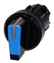
Selector switch, illuminable, 22 mm, round, plastic, blue, selector switch, short, 3 switch positions I>O<II, momentary contact type, actuating angle  $2x45^{\circ}$ , 10:30h/12h/13:30h, with laser labeling, lower case
