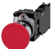
Mushroom pushbutton, 22 mm, round, metal, shiny, red, 40mm, latching, pull-tounlatch mechanism, with holder, 1 NO+1 NC, spring-type terminal, with laser labeling, upper case
