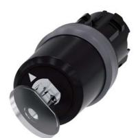
Key-operated switch BKS, 22 mm, round, plastic with metal front ring, lock No. E9 (VW), without key, 2 switch positions O-I, latching, actuating angle  $90^{\circ}$ , 10:30h/13:30h, key removal O+I, with laser labeling, upper case and lower case, always upper case at the beginning of the word
