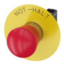
EMERGENCY STOP mushroom-type actuator, 22 mm, round, metal, shiny, red, 40 mm, positive latching, according to EN ISO 13850, rotate-to-unlatch, with yellow backing plate, inscription: NOT-HALT, with holder, 1 NC, spring-type terminal
