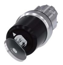
Key-operated switch BKS, 22 mm, round, metal, shiny, Lock No. E9 (VW), without key, 2 switch positions O-I, latching, actuating angle 90°, 10:30h/13:30h, key removal O, with laser labeling, lower case
