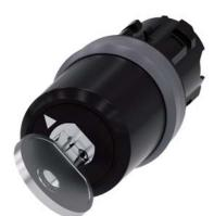
Key-operated switch BKS, 22 mm, round, plastic with metal front ring, special lock, with 2 keys, 2 switch positions O-I, latching, actuating angle 90°, 10:30h/13:30h, key removal O, Note: BKS locking systems E1 - E25 supplied without key
