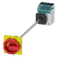
Load disconnector 3LD3, Iu 40 A Main switch 3-pole + N Rated operating capacity at AC-23 A at 400 V 18.5 kW floor mounting Basic switch with door coupling Central hole mounting 22.5mm Rotary actuator red / yellow 66 x 66 mm
