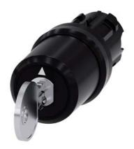
Key-operated switch BKS, 22 mm, round, plastic, lock number S1, with 2 keys, 3 switch positions I>O<II, momentary contact type, actuating angle  $2x45^\circ, 10:30h/12h/13:30h,$  key removal O, with laser labeling, lower case
