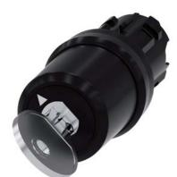
Key-operated switch BKS, 22 mm, round, plastic, Lock No. E2 (VW), without key, 2 switch positions O-I, latching, actuating angle  $90^{\circ}$ , 10:30h/13:30h, key removal O+I, with laser labeling, upper case
