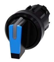
Selector switch, illuminable, 22 mm, round, plastic, blue, selector switch, short, 3 switch positions I-O<II, left latching, right momentary contact type, actuating angle  $2x45^{\circ}$ , 10:30h/12h/13:30h, with laser labeling, upper case
