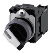
Selector switch, illuminable, 22 mm, round, plastic with metal front ring, white, selector switch, short, 2 switch positions O-I, latching, actuating angle  $90^\circ,\,10:\!30h/13:\!30h,$  with holder, 1 NO, Z=20-unit packaging
