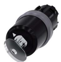
key-operated switch Siemens, 22 mm, round, plastic with metal front ring, lock no. LSG1, with 2 keys, 2 switch positions O<I, momentary contact type, actuating angle  $45^{\circ}$ , 10:30h/12h, key removal O
