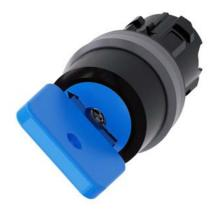
Key-operated switch O.M.R, 22 mm, round, plastic with metal front ring, lock number 73038, blue, with 2 keys, 2 switch positions O-I, latching, actuating angle 90°, 10:30h/13:30h, key removal O+I, with laser labeling, upper case and lower case, always upper case at the beginning of the word
