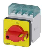
SENTRON, Switch disconnector 3LD, emergency switching-off switch, 4- pole, lu: 16 A, operating power / at AC-23 A 400 V: 7.5 kW, front-mounted, knob-operated mechanism, red/yellow, 4-hole mounting of the handle
