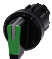
Selector switch, illuminable, 22 mm, round, plastic, green, selector switch, short, 3 switch positions I-O-II, latching, actuating angle 2x45°, 10:30h/12h/13:30h, with laser labeling, lower case
