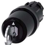
Key-operated switch IKON, 22 mm, round, plastic, lock number 360012K1, with 2 keys, 3 switch positions I>O<II, momentary contact type, actuating angle 2x45°, 10:30h/12h/13:30h, key removal O, with laser labeling, upper case and lower case, always upper case at the beginning of the word
