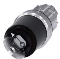
Key-operated switch IKON, 22 mm, round, metal, shiny, lock number 360012K1, with 2 keys, 2 switch positions O-I, latching, actuating angle  $90^{\circ}$ , 10:30h/13:30h, key removal O, with laser labeling, upper case
