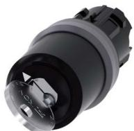
Key-operated switch IKON, 22 mm, round, plastic with metal front ring, lock number 360012K1, with 2 keys, 2 switch positions O-I, latching, actuating angle 90°, 10:30h/13:30h, Key removal O+I
