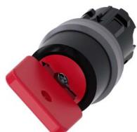
Key-operated switch O.M.R, 22 mm, round, plastic with metal front ring, lock number 73037, red, with 2 keys, 2 switch positions O-I, latching, actuating angle 90°, 10:30h/13:30h, key removal O+I, with laser labeling, inscription or symbol Customer-specific selection with SIRIUS ACT configurator (CIN)
