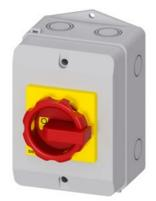
SENTRON, Switch disconnector 3LD, emergency switching-off switch, 4- pole, 32 A, operating power at AC-23 A at 400 V: 11.5 kW, molded-plastic encapsulation for metric cable gland, rotary operating mechanism, red/yellow
