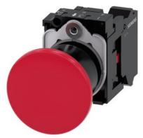
Mushroom pushbutton, 22 mm, round, plastic, red, 40mm, latching, pull-to-unlatch mechanism, with holder, 1 NC, spring-type terminal, Z=20-unit packaging
