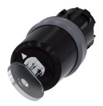
Key-operated switch BKS, 22 mm, round, plastic with metal front ring, Lock number E1 (VW), without key, 2 switch positions O-I, latching, actuating angle  $90^\circ$ , 10:30h/13:30h, key removal O, with laser labeling, upper case
