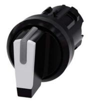
Selector switch, illuminable, 22 mm, round, plastic, white, selector switch, short, 3 switch positions I>O<II, momentary contact type, actuating angle 2x45°, 10:30h/12h/13:30h, with laser labeling, upper case and lower case, always upper case at the beginning of the word
