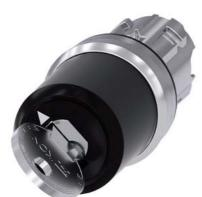
Key-operated switch IKON, 22 mm, round, metal, shiny, special lock, with 2 keys, 2 switch positions O-I, latching, actuating angle  $90^{\circ}$ , 10:30h/13:30h, Key removal O
