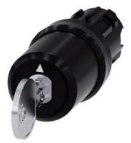
Key-operated switch BKS, 22 mm, round, plastic, special lock, with 2 keys, 3 switch positions I>O<II, momentary contact on the left, latching on the right, actuating angle  $2x45^\circ, 10:30h/12h/13:30h,$  key removal O, Note: BKS locking systems E1 - E25 supplied without key
