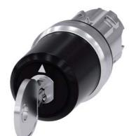
key-operated switch Siemens, 22 mm, round, metal, shiny, special lock, with 2 keys, 3 switch positions I-O-II, latching, actuating angle  $2x45^{\circ}$ , 10:30h/12h/13:30h, key removal I
