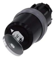
Key-operated switch BKS, 22 mm, round, plastic with metal front ring, lock No. E9 (VW), without key, 2 switch positions O-I, latching, actuating angle  $90^\circ, 10:30h/13:30h,$  key removal O, with laser labeling, upper case and lower case, always upper case at beginning of line
