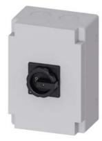
SENTRON, Switch disconnector 3LD, main switch, 3-pole, lu: 125 A, Operating power / at AC-23 A at 400 V: 45 kW, molded-plastic encapsulation for inch cable gland, rotary operating mechanism, black
