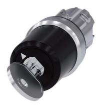
Key-operated switch BKS, 22 mm, round, metal, shiny, Lock No. E9 (VW), without key, 2 switch positions O-I, latching, actuating angle 90°, 10:30h/13:30h, key removal O, with laser labeling, upper case and lower case, always upper case at the beginning of the word
