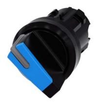
Selector switch, illuminable, 22 mm, round, plastic, blue, selector switch, short, 2 switch positions O<I, momentary contact type, Actuating angle 45°, 10:30h/12h, with laser labeling, upper case and lower case, always upper case at beginning of line
