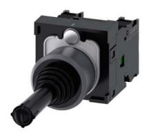
Coordinate switch, 22 mm, round, plastic with metal front ring, black, 2 switch positions, horizontal, momentary contact type, without mechanical interlocking in O position, with holder, 1 NO, 1 NO, screw terminal, Z=20-unit packaging
