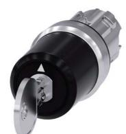
Key-operated switch BKS, 22 mm, round, metal, shiny, lock number S1, with 2 keys, 3 switch positions I>O<II, momentary contact type, actuating angle 2x45°, 10:30h/12h/13:30h, key removal O, with laser labeling, upper case and lower case, always upper case at the beginning of the word
