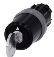
Key-operated switch BKS, 22 mm, round, plastic with metal front ring, lock number S1, with 2 keys, 3 switch positions I-O-II, latching, actuating angle  $2x45^{\circ}$ , 10:30h/12h/13:30h, key removal II
